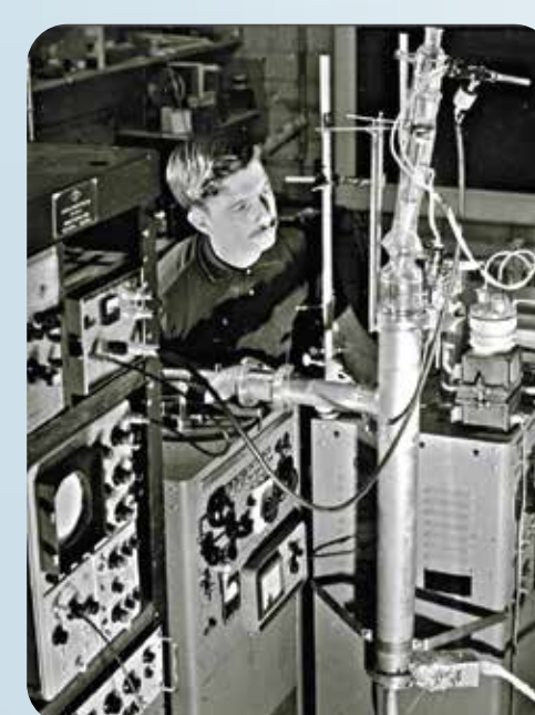
Erwin W. Müller John A. Panitz Introduce the Atom-Probe Field Ion Microscope (APFIM) 1967
