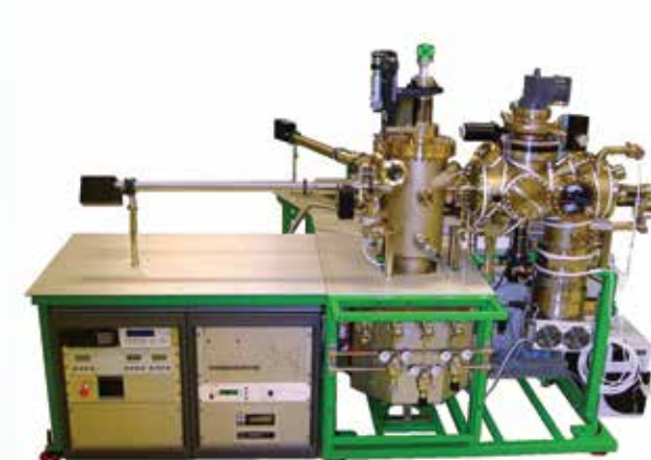
Tomographic Atom Probe Didier Blavette et al. Second 3D Atom Probe with an improved detector 1990
