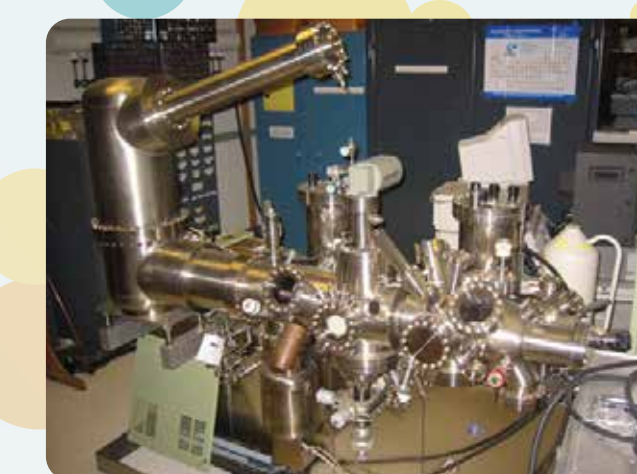
1984 Vacuum Generators, APFIM 100 with help from G.D.W. Smith Group First shipped commercial atom probe
