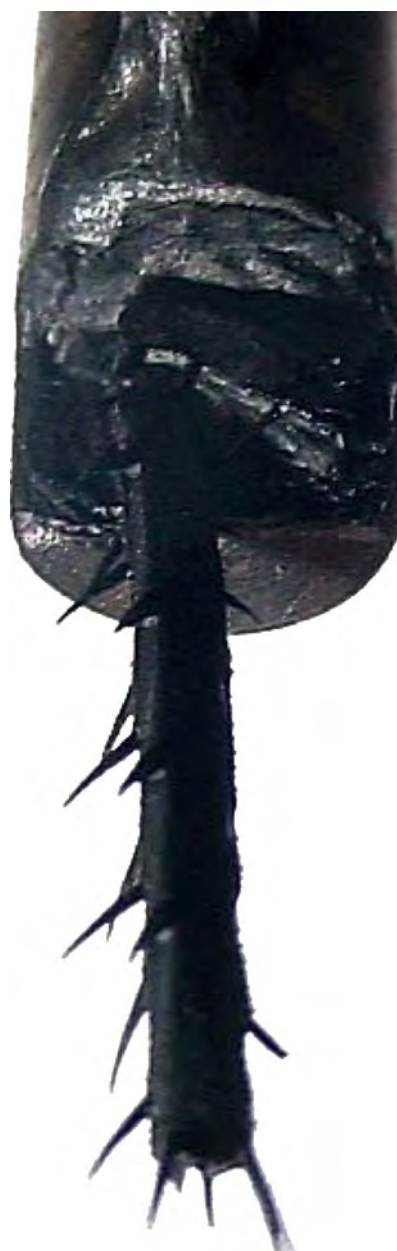
Fig. 4. A biological sample. A cockroach leg was attached to a brass rod (0.5 cm in diameter) with a colloidal silver liquid and spray coated with a graphite dispersion in isopropyl alcohol to make it conductive.
