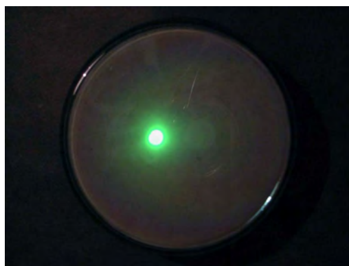
Fig. 7. A focused electron beam. About 0.5 A is applied to the electron lens.
