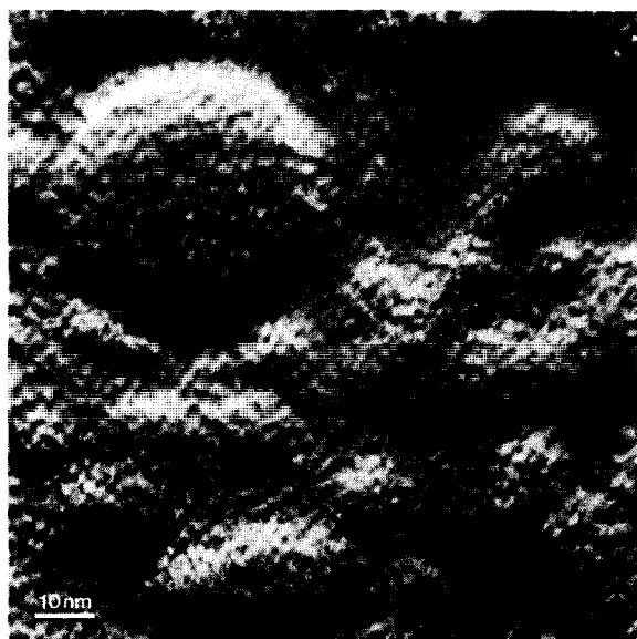
Fig. 6. The same reconstruction as shown in fig. 4 with three additional images (corresponding to greater distances from the tip surface) included in the digital sum. A comparison of this image with that shown in fig. 4 indicates that the additional images have the effect of developing the morphology of the large circular features while leaving the other image feature intact.
