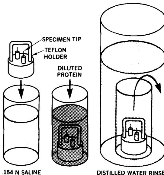
Fig. 1. A schematic drawing of the aqueous dosing procedure developed to place biomolecules on large radius field-emitter tips.
