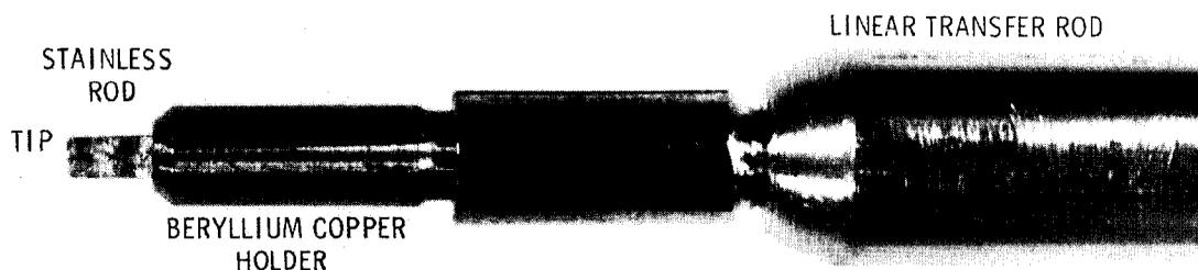
FIG. 4. The tip holder and transfer rod. The specimen "tip" is spot welded to a stainless steel support rod (extreme left) flattened to facilitate spot welding and inserted into a beryllium copper holder. This holder plugs into a second beryllium copper holder, which is mounted at the end of the linear transfer rod.
