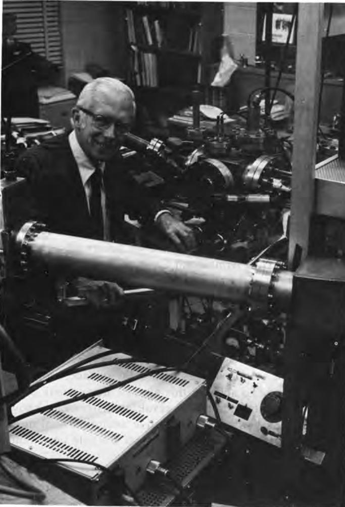
Erwin W. Mueller with his energy focused time-of-flight Atom-Probe Field Ion Microscope.
