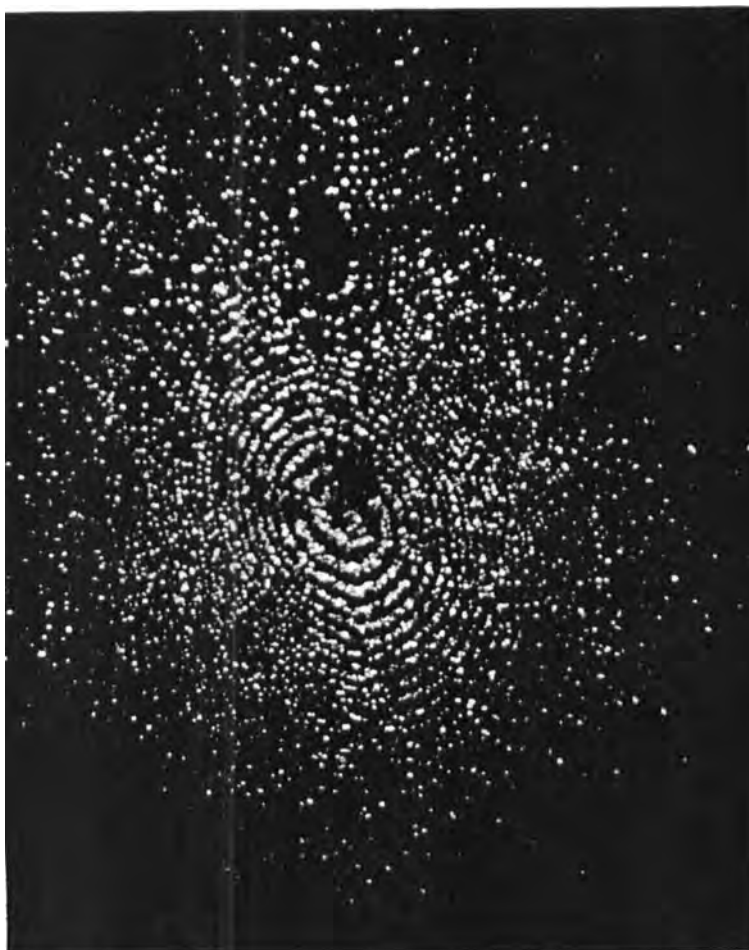
FIGURE 8. Desorption micrograph of tungsten at 78 K. Dark spot (above center of 110 plane) is a detector anomaly. (Micrograph courtesy of Dr. R. J. Walko, The Pennsylvania State University, now at Sandia Laboratories.)
