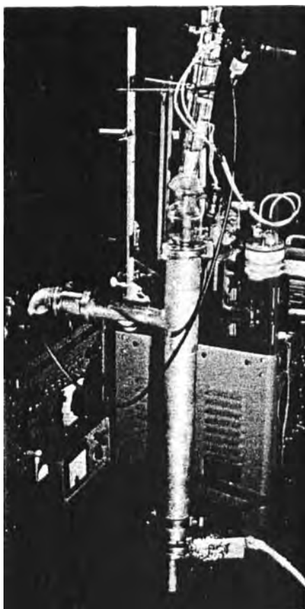
FIGURE 1A. The original atom-probe field-ion microscope. The glass specimen chamber is uppermost, with a spherical grease joint providing specimen movement. The separately pumped drift tube is 1 m long.
