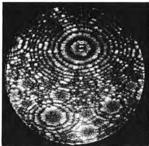
FIGURE 12. Helium-ion image of (110) tungsten (right). Integrated W^{++} image (middle), 100 desorption events in 100 sec. Integrated W^{++} image (left), 100 desorption events in 100 sec. P \approx 8 \times 10^{-10} torr, T = 78 K.
